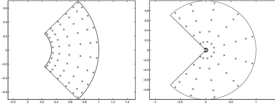
Figure 2:  $60 = 6 \times 10$  product quadrature nodes of algebraic exactness degree 9 on circular sectors with  $R_1 = 1/3$ ,  $R_2 = 1$ ,  $\omega = \pi/4$  (left) and  $R_1 = 0$ ,  $R_2 = 1$ ,  $\omega = 3\pi/4$  (right).
