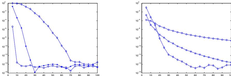
Figure 5: Relative errors in the integration of two parametric functions on the circular segment (15) ( $\alpha = 0$ ), with  $R = 1$  and  $\beta = \pi/3$ , for  $n = 5, 10, 15, \dots, 95, 100$ ; left:  $f(x, y) = \exp(k(x + y))$ ,  $k = 1$  ( $\circ$ ),  $k = 10$  ( $*$ ),  $k = 100$  ( $\diamond$ ); right:  $f(x, y) = \exp([(x - a)^2 + (y - b)^2]^{5/2})$ ,  $(a, b) = (0.7, 0)$  ( $\circ$ ),  $(a, b) = (1, 0)$  ( $\square$ ),  $(a, b) = (1/2, \sqrt{3}/2)$  ( $\diamond$ ).
