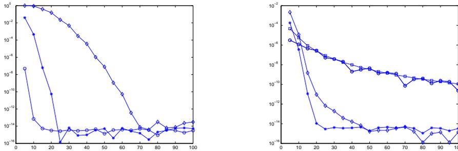
Figure 3: Relative errors in the integration of two parametric functions on the sector (13) with  $R = 1$  and  $\omega = \pi/3$ , for  $n = 5, 10, 15, \dots, 95, 100$ ; left:  $f(x, y) = \exp(k(x+y))$ ,  $k = 1$  ( $\circ$ ),  $k = 10$  ( $*$ ),  $k = 100$  ( $\diamond$ ); right:  $f(x, y) = \exp([(x-a)^2 + (y-b)^2]^{5/2})$ ,  $(a, b) = (0.3, 0)$  ( $\circ$ ),  $(a, b) = (1, 0)$  ( $\square$ ),  $(a, b) = (1/2, \sqrt{3}/2)$  ( $\diamond$ ),  $(a, b) = (0, 0)$  ( $*$ ).
