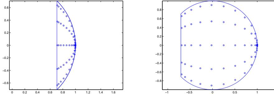
Figure 4:  $60 = 5 \times 12$  product quadrature nodes of algebraic exactness degree 9 on circular segments (15) ( $\alpha = 0$ ), with  $R = 1$  and  $\beta = \pi/4$  (left),  $\beta = 3\pi/4$  (right).
