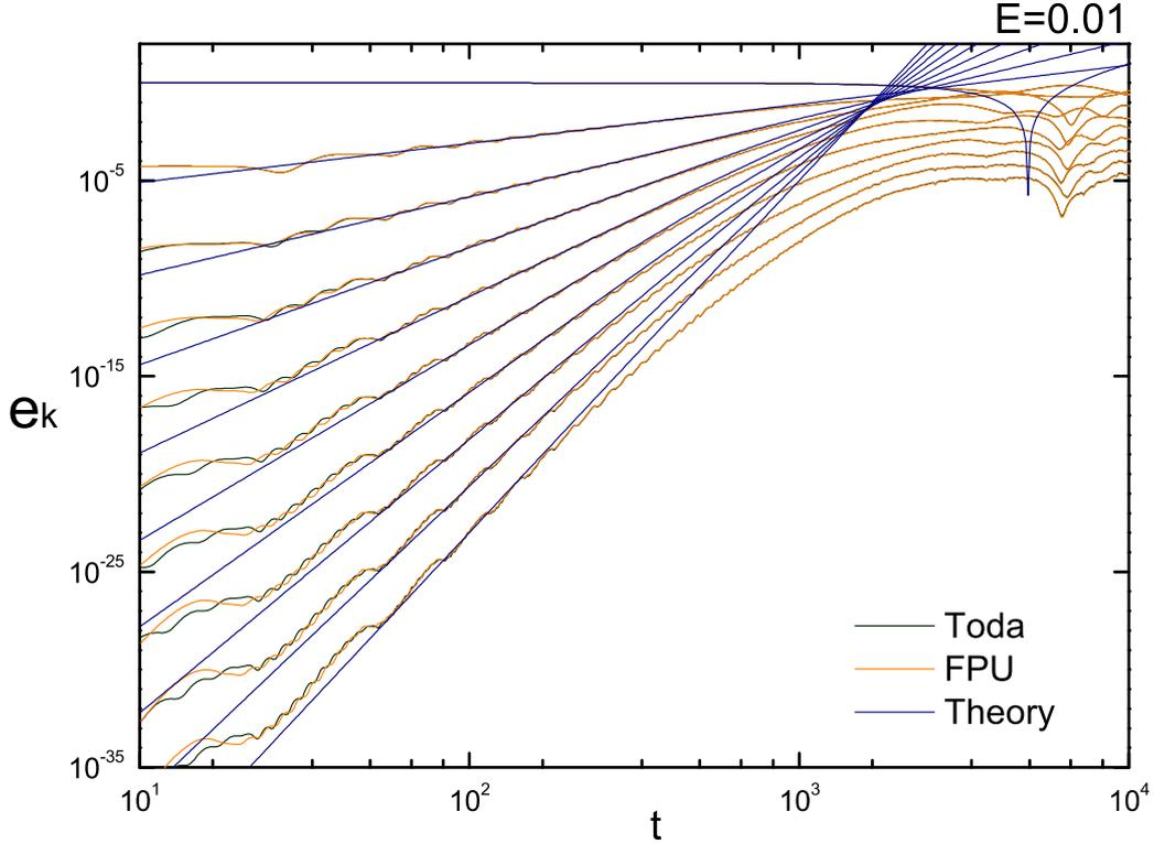
FIG. 2.  $e_k(t)$  vs.  $t$  (log-log scale) for  $k = 1, \dots, 10$  at  $E = 0.01$ ; black and orange curves refer respectively to the Toda and the FPU numerically computed energies, while blue lines correspond to the theoretical law (11)-(12).
