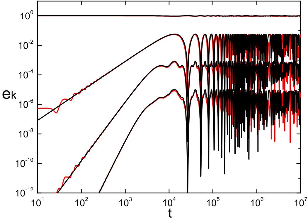
FIG. 11.  $e_k$  vs.  $t$  (log-log scale),  $k = 1, 2, 3, 4$ , for FPU,  $E = 10^{-4}$ . Red curves: numerical data. Black curves: analytic prediction.
