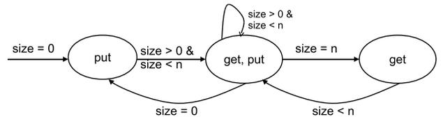
Figure 5: Bounded Buffer State Diagram
