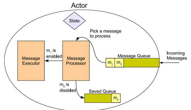
Figure 6: Implementation semantics of local synchronization constraints in ActorFoundry
