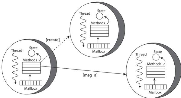
**Figure 1: Actors are concurrent entities that exchange messages asynchronously.**
