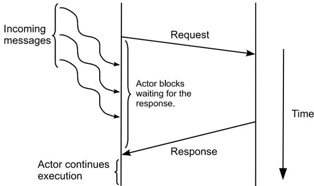
Figure 4: Request-reply messaging pattern blocks the sender of a request until it receives the reply. All other incoming messages during this period are deferred for later processing.
