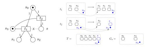
Figure 10. A reset Petri net and the corresponding SPO grammar.
