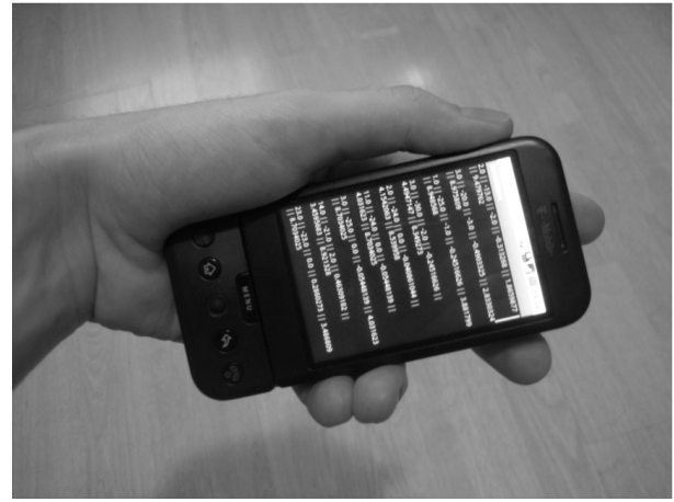
Fig. 5. An experimental session with DroidGlove implemented on a HTC G1 smartphone: debug information about acceleration and orientation is reported in real-time on the screen.
