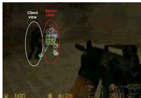
Figure 2. Frame sequence of a game session as seen by a client: other participants are positioned in the game arena with a lag that depends on the distance between clients and server.
