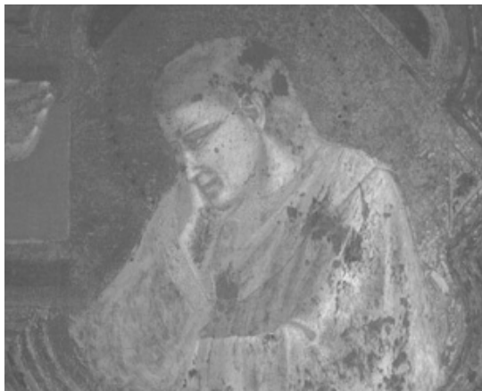
Figure 3. Visible Fluorescence Image of Giotto's Crucifix; Detail of Saint John. Numerous Retouches (Black Areas) Are Visible on Saint John's Head and Dress.
