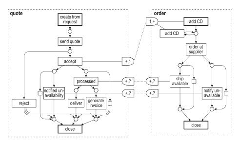
Fig. 1. A proclet system describing the back-end process of a CD online shop. A customer's quote is split into several orders according to the suppliers of the CDs; an order at a supplier handles several quotes from different customers.
