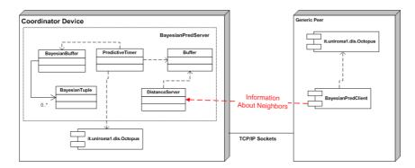
Figure 5: The components of the actual implementation.
