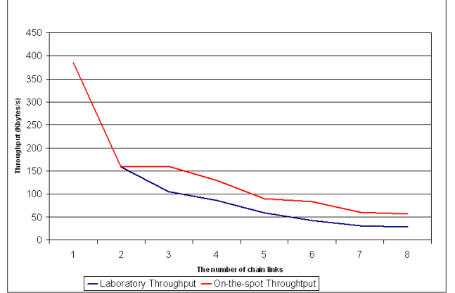
Figure 2. Test results for a chain-MANET, in the laboratory and estimated on-the-spot results
