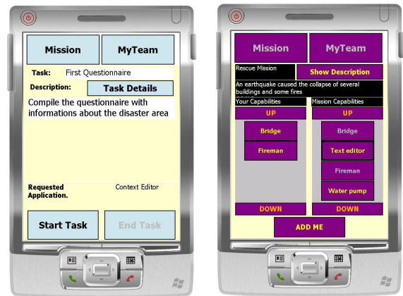
(c) When the engine decides to assign a non-automatic task to a certain human participant, she is informed through Task Handler. Then, by clicking on button "Start Task", the application to execute that task is launched.
