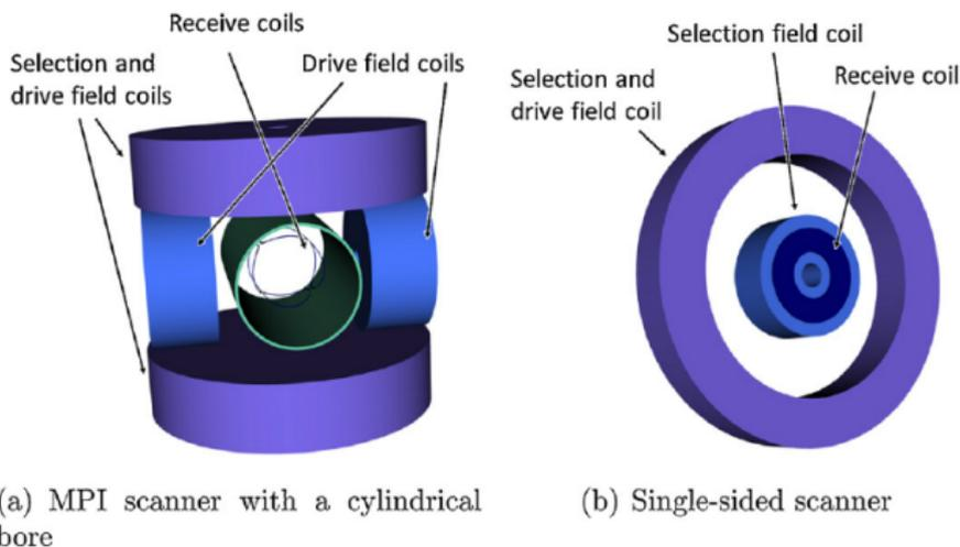
**Figure:** **Left:** two pairs of transmit coils and two pairs of receivers coils.
