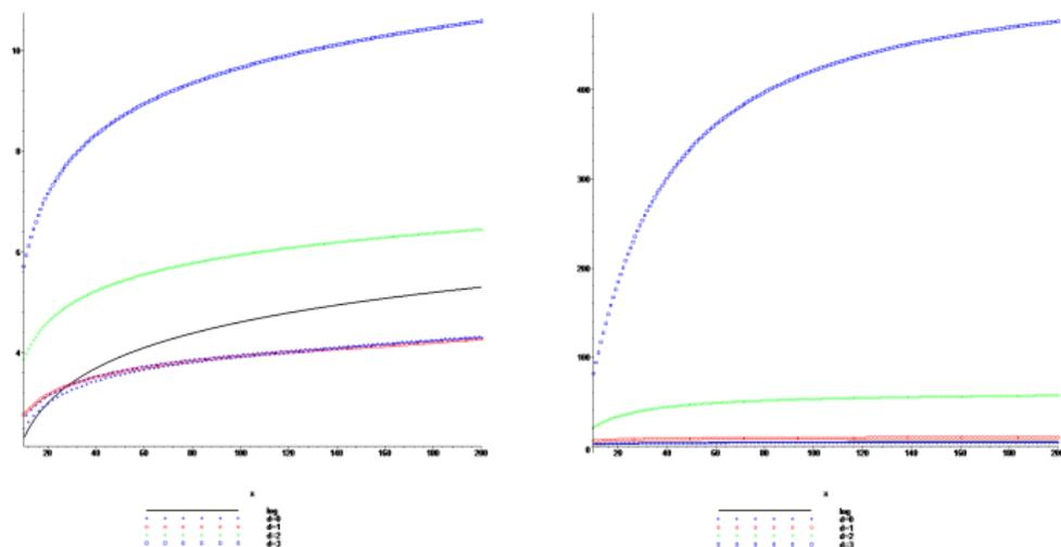
**Figure:** Lebesgue constant on logarithmically distributed points. **Left:** with weights  $(-1)^i \beta_j$ . **Right:** here the weights are the ones constructed on non-equispaced points, guaranteeing the approximation order  $d+1$
