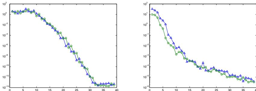
Figure 2: Uniform error (circles) and estimate (10) (triangles) of Newton interpolation at Discrete Leja Points on the square for  $\nu = 2, \dots, 40$ ; Left:  $f(x_1, x_2) = \cos(5(x_1 + x_2))$ ; Right:  $f(x_1, x_2) = [(x_1 - 1/3)^2 + (x_2 - 1/3)^2]^{5/2}$ .
