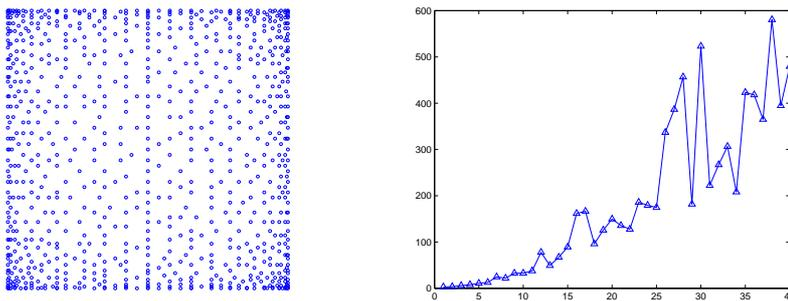
Figure 1: Left:  $N = 861$  Discrete Leja Points for degree  $n = 40$  on the square, extracted from an  $81 \times 81$  Chebyshev-Lobatto grid; Right: Lebesgue constants of Discrete Leja Points on the square for  $n = 1, \dots, 40$ .
