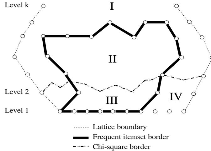
**Fig. 1.** Lattice structure for all itemsets. This structure can be divided into several regions : I. Infrequent and dependent itemsets, II. frequent and dependent itemsets, III. frequent and independent itemsets, IV. infrequent and independent itemsets.
