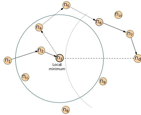
Fig. 2. GFG algorithm over a 2-D graph. Solid arrows represent greedy-mode forwarding and dashed arrows represent face-mode forwarding.
