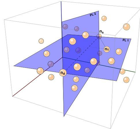
Fig. 3. In AB3D, plane  $PL_1$  passes through  $n_s$ ,  $n_d$ , and  $n_1$ , and plane  $PL_2$  is orthogonal to  $PL_1$ . Both planes contain the line  $(n_s n_d)$ .
