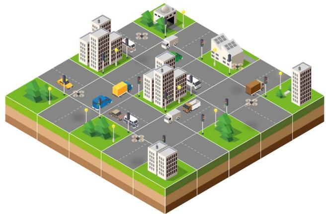
Fig. 8. Multitier IoV network comprised of moving cars, drones, and traffic intersections equipped with sensing and communication capabilities. In this envisaged scenario communication takes place amongst entities in a multihop fashion. Cars could exploit the IoV sensing capabilities, gathering and merging information from different complementary sources in order to extend the drivers' perception beyond direct line of sight.
