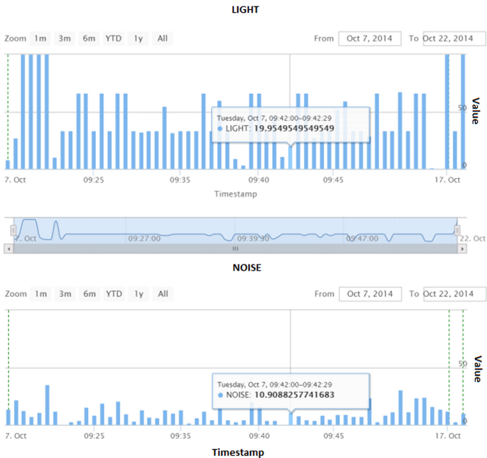
Fig. 10. Histogram charts showing brightness and noise values along time.
