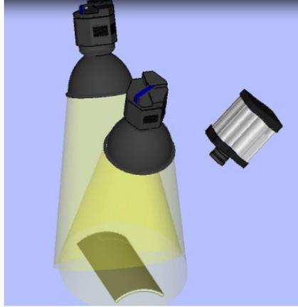
**Figure 8.1:** *Infrared thermographic inspection: in the time interval  $[0, t_f]$ ,  $t_f > 0$ ,  $S$  is heated with a thermal flash  $\mathbf{q}(t)$  and experimental temperatures are collected.*
