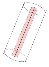
Fluid dragged along the axial direction by the inner cylinder, adherence at  $R_1$  and  $R_2$ .
