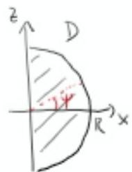
$$\begin{aligned} \text{Volume} &= 2\pi \int_D x \, dx \, dz = 2\pi \int_{-\pi/2}^{\pi/2} d\psi \int_0^R \int_0^R \sin\psi \cdot \rho \, d\rho \, dz \\ &= 2\pi \int_{-\pi/2}^{\pi/2} \sin\psi \, d\psi \int_0^R \rho^2 \, d\rho = (\sin\psi) \Big|_{-\pi/2}^{\pi/2} \cdot \left(\frac{\rho^3}{3}\right) \Big|_0^R = 2\pi \cdot 2 \cdot \frac{R^3}{3} = \frac{4\pi}{3} R^3 \end{aligned}$$
