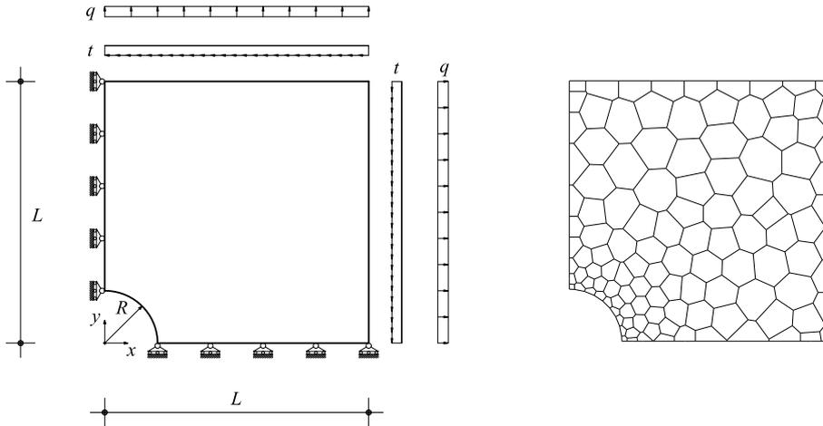
Figure 5: Infinite plate with hole. Left: geometry, boundary conditions, loading for the computational domain. Right: representative Voronoi tessellation for VEM analysis.
