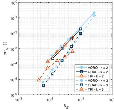
Figure 8: Asymptotic homogenization.  $H^1$  error norm *vs* mesh size  $h_E$  for  $k = 2$  and  $k = 3$  VEM approximations of the homogenization problem.
