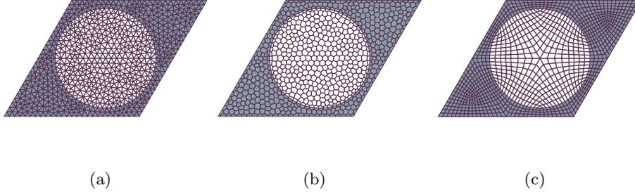
Figure 7: Asymptotic homogenization. Parallelogram unit cell with circular inclusion ( $v_f = 0.5$ .) Representative mesh types. (a) Tri-mesh. (b) Voro-mesh. (c) Quad-mesh
