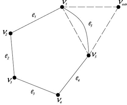
Figure 2: **Typical curvilinear virtual element (case  $k = 1$ ) at fibre matrix curved interface boundary. Case with curved edge no. 5 equipped with additional degree of freedom (node  $v_{extra}$ ).**
