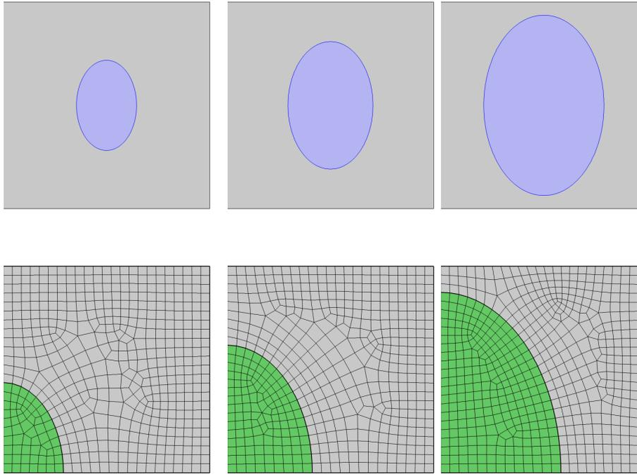
Figure 11: Asymptotic homogenization of doubly periodic composite material with elliptical inclusions. Square RUC, volume fraction  $f = \{0.1, 0.2, 0.4\}$  (*upper panel*), stiffness contrast factor  $\xi = 50$ , perfect interface s.t.  $\delta = \infty$ . Curvilinear quadrilateral meshes of a relevant quarter of domain due to double symmetry with respect to  $(y_1, y_2)$  axes (*lower panel*). Elliptical inclusion semi-axis ratio equal to  $2/3$ .
