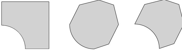
Figure 3: Some domains  $\mathcal{S}$  of polygonal type in which a side is substituted by a circular arc. In all these examples  $\partial\mathcal{S}$  is locally a  $p$ -th degree NURBS curve.
