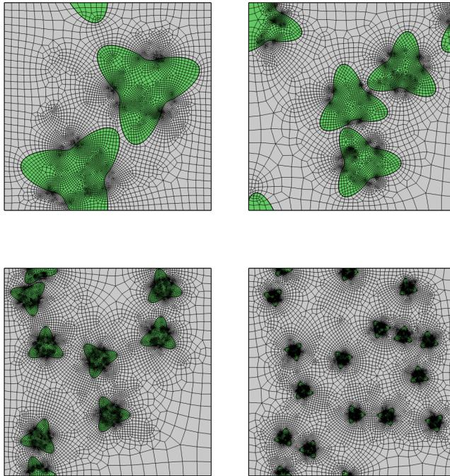
Figure 15: Statistic homogenization of a composite with randomly distributed fibres with complex curvilinear cross section geometry. Stochastic realization of a square RUC of a composite with prescribed volume fraction  $f = 0.2$  and respectively 2, 3, 4, 16 complex shaped trilobed fibres: conforming curvilinear quadrilateral meshes.
