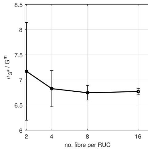
Figure 16: Statistic homogenization of a composite with randomly distributed fibres with complex curvilinear cross section geometry. Mean value  $\mu_{G^{\#}}$  and dispersion of  $G^{\#}$ , normalized by  $G^m$  as a function of the number of trilobe inclusion per RUC obtained through Monte Carlo simulation; fibre/matrix stiffness ratio  $\xi = 1000$ . , perfect interface ( $\delta = \infty$ ).
