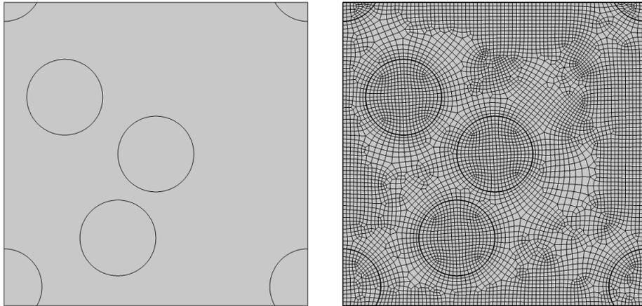
Figure 1: Stochastic realization of a square-shaped repeating unit cell (RUC) of a composite with volume fraction  $f = 0.2$  and four circular fibres (*left panel*). Conforming curvilinear quadrilateral mesh (*right panel*).
