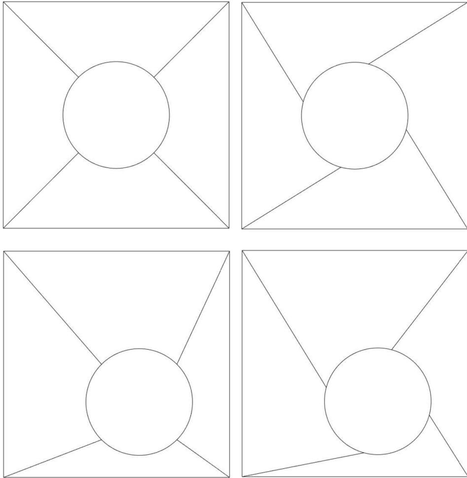
Figure 9: Patch test on a unit square domain. Minimal curvilinear polygon meshes comprising a quadrilateral with four convex circular edges with same radius and four quadrilaterals with one concave circular edge. Meshes are progressively distorted through shift and rotation of inner polygon.
