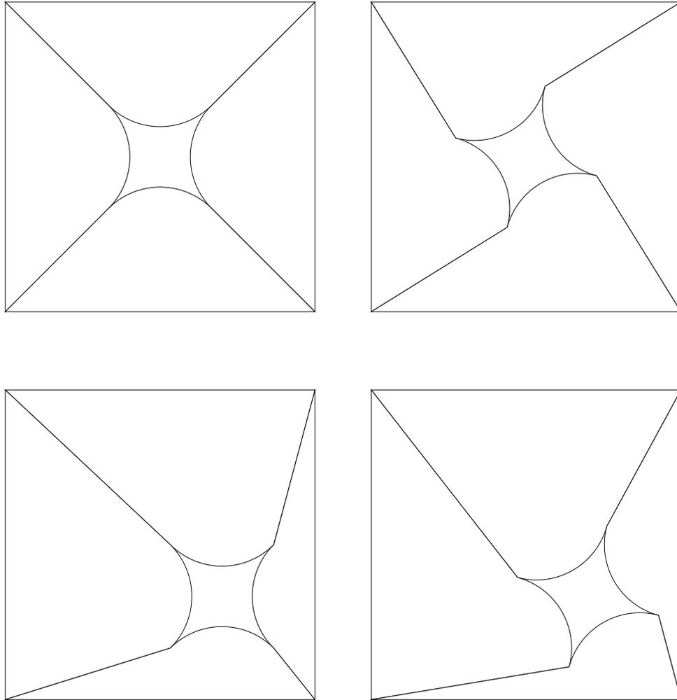
Figure 10: Patch test on a unit square domain. Minimal curvilinear polygon meshes comprising a quadrilateral with four concave circular edges with same radius and four quadrilaterals with one convex circular edge. Meshes are progressively distorted through shift and rotation of inner polygon.
