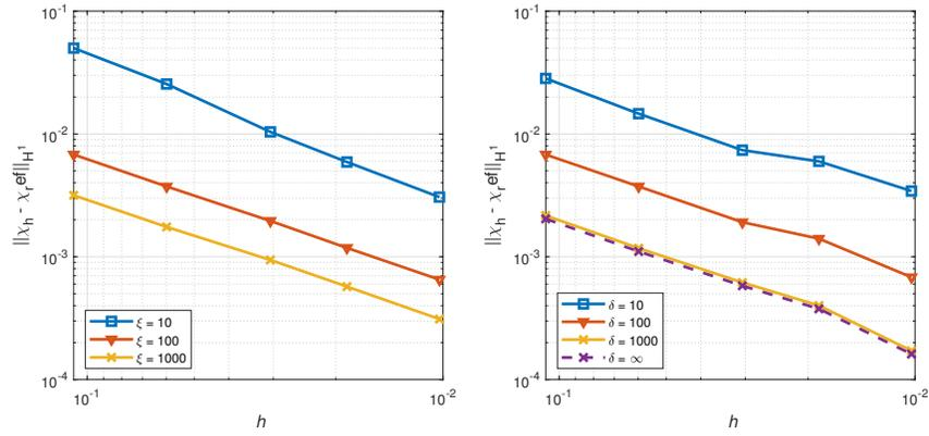
Figure 14: Asymptotic homogenization of doubly periodic composite material with complex bi-lobe inclusions.  $h$ -convergence in the  $H^1$  error norm on the cell function  $\chi$  for varying stiffness contrast factor  $\xi$  (left panel), and varying interface parameter  $\delta$  (right panel).
