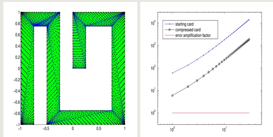
Left: the 14415 blue quadrature points are the support of an algebraic quadrature rule of degree 60. The 1891 black points, extracted by quadratic programming, fits the moments up to an absolute error of  $1.2215 \cdot 10^{-14}$ .
