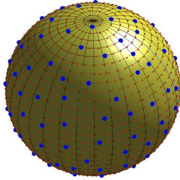
Figure 1: CATCH submesh (121 points, bullets) extracted by NNLS from a zonal equal area mesh (1265 points, dots) of the sphere for degree  $n = 5$ .
