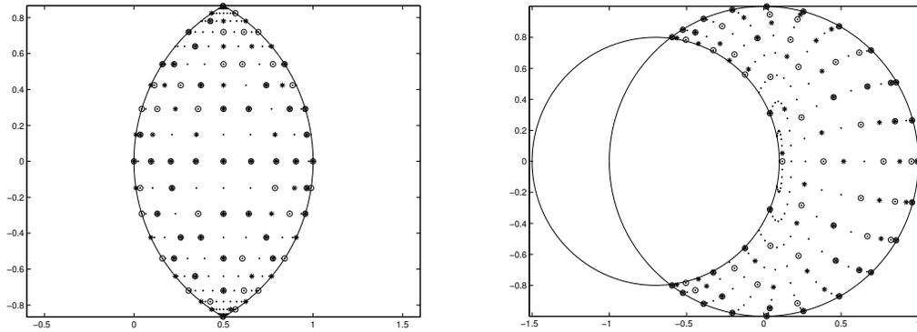
Figure 2: 66 Approximate Fekete Points (o) and Discrete Leja Points (\*) extracted from a WAM (·) for degree  $n = 10$  on a symmetric lens (left) and on a lune (right).
