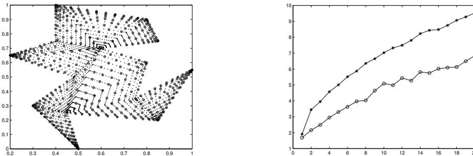
Figure 1: Left: WAM for degree  $n = 15$  ( $\cdot$ , about 2800 points) by triangulation on a polygon with 14 sides, and its compression into  $496 = \dim(\mathbb{P}_{2n}^2)$  points ( $\circ$ ); Right: Lebesgue constants of the LS operator on the original ( $*$ ) and the compressed WAM ( $\circ$ ),  $n = 1, \dots, 20$ .
