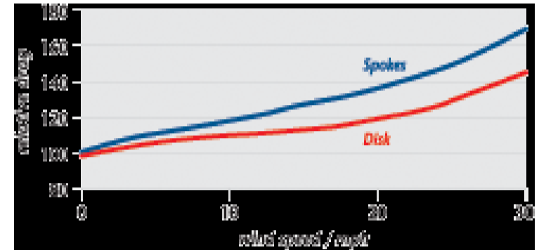
Graph of relative drag difference between a cyclist using a rear wheel with and without a disk in a range of crosswinds
