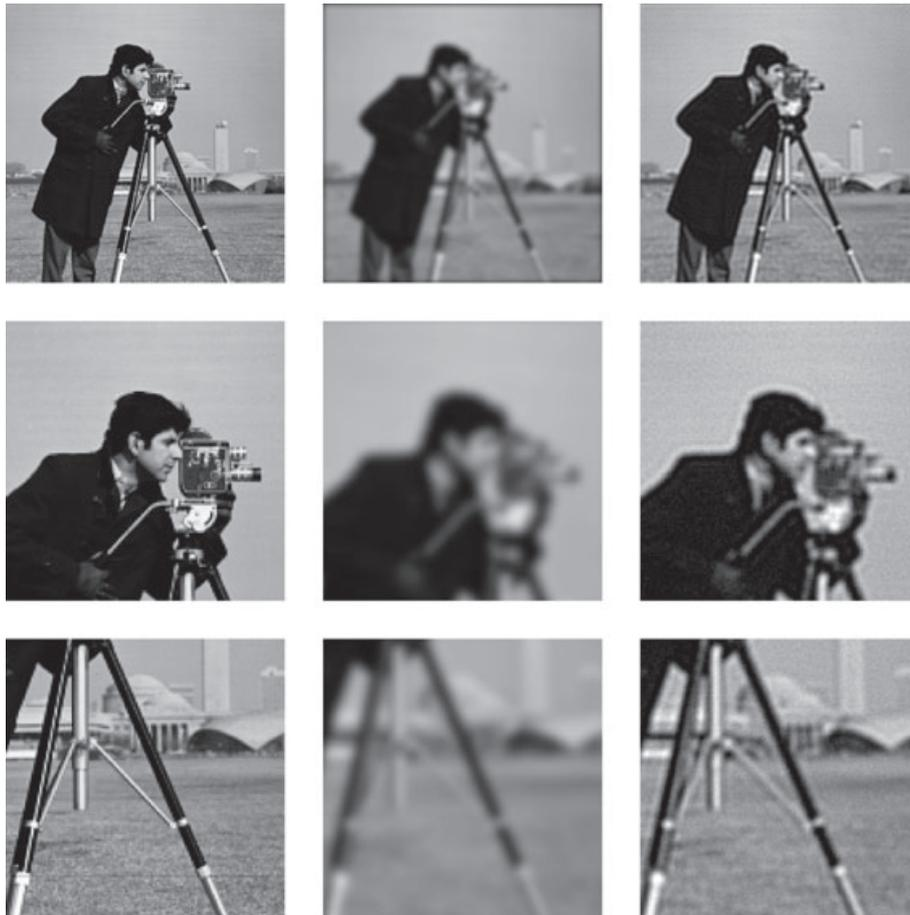
Figure 8. Restoration of `cameraman.tif`. From left to right: original image; blurred and noisy image with blur parameters `band = 7`, `sigma = 2`, and noise level  $\varepsilon = 10^{-3}$ ; and restored image. From top to bottom: original size image and two zooms.
