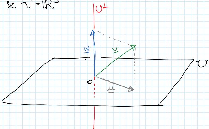
$$\underline{u}_1 = P_U(\underline{v}) = \text{PROIEZIONE ORTOGONALE DI } \underline{v} \text{ SU } U$$
