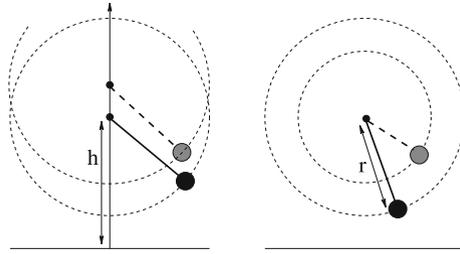
**Fig. 1.** *Left* a pendulum with vertically moving pivot and fixed length. *Right* a pendulum with fixed pivot and variable length
