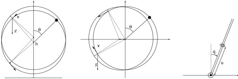
**Fig. 3.** A pendulum whose pivot oscillates vertically (on the left) and horizontally (center). On the right: a bead sliding without friction along a rotating axis
