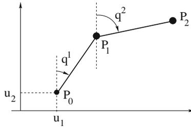
**Fig. 4.** Controlling a double pendulum by moving the pivot at  $P_0$
