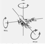
Any three-dimensional rotation can be described as a sequence of *roll* (*x*), *pitch* (*y*), *yaw* (*z*) rotations (Euler angles)
