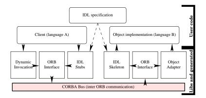
The IDL specifies modules, constants, types and interfaces. An object interface defines the operations, exceptions and public attributes a client can invoke or access. CORBA offers a model based only on distributed objects. In some respects, it can be compared to Java as this language provides only an object-oriented programming model, and discards the classical structured programming model.
