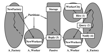
When a worker has completed his job, the result must be saved in a common storage. To do this, we define a protected area in SP package Storage (see following code). An entry-less protected object ensures atomic access to this area.
